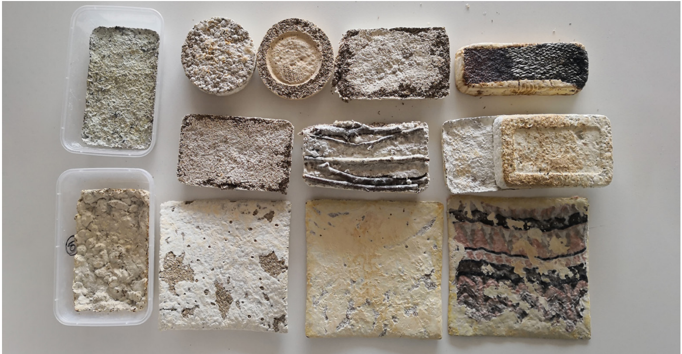
Image: Mycelium-composite growth tests, various substrates; University of Tasmania.
