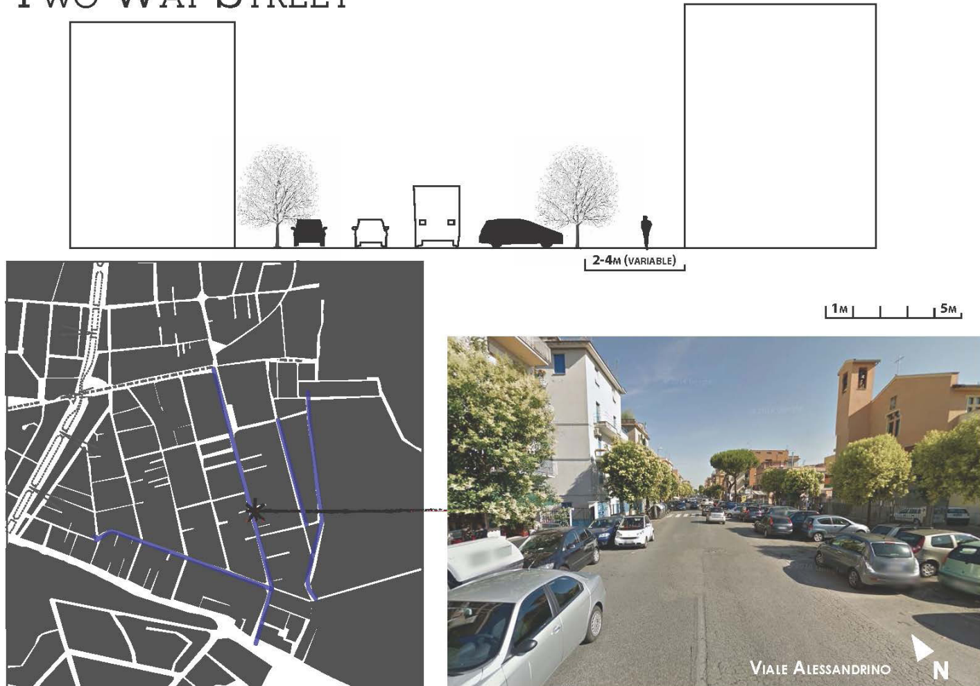
Figure 22. Two way primary street section
